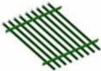
Fig.4 Repeat instructions in Fig.2 and slide the two cross members towards one another up to the point of the dimples on the pales.
