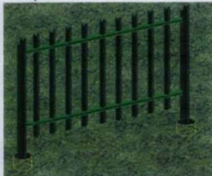
Fig.12 Two metre section is secured in the ground with concrete and is now tamper proof.
