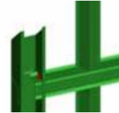
Fig.8 The post is now ready to have the extended pale secured in designated groove.
