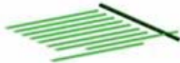
Fig.1 Nine pales are laid on the ground. Place one cross member across the top and one across the bottom.
